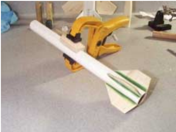
Figure 4-7 – Attaching the Glider Mounting Saddle
