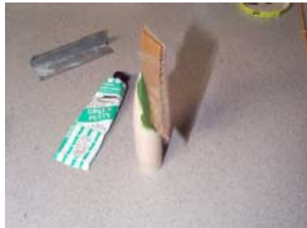
Figure 4-11 – Filling the Nose Cone Slot
