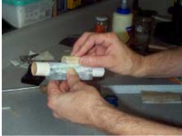
Figure 4-8 – Sanding the Glider Saddle BT-50 Contour
