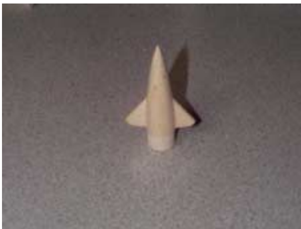
Figure 3-10 – Nose Cone and Canards
