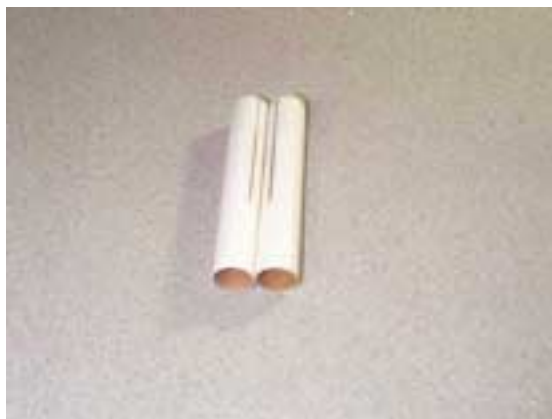
Figure 3-2 – Nacelle Halves Assembled and Drying
