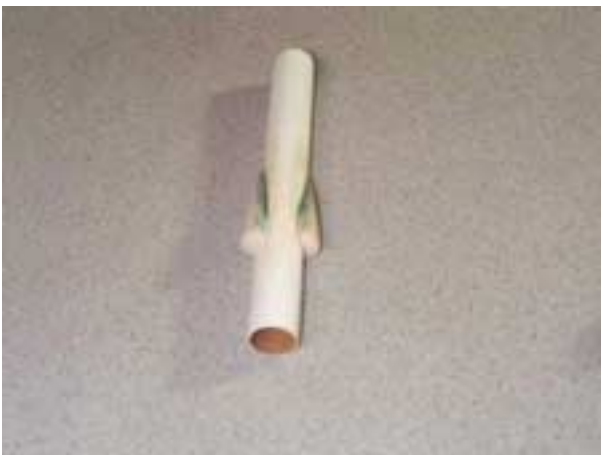
Figure 3-5 – Air Intakes Filleted and Ready to Prime
