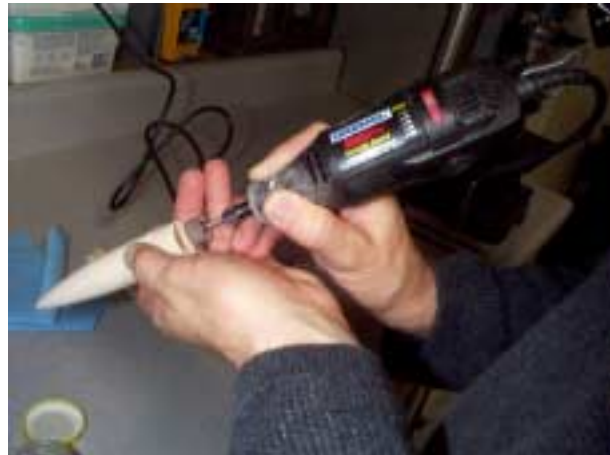
Figure 4-9 – Hollowing the Nose Cone
