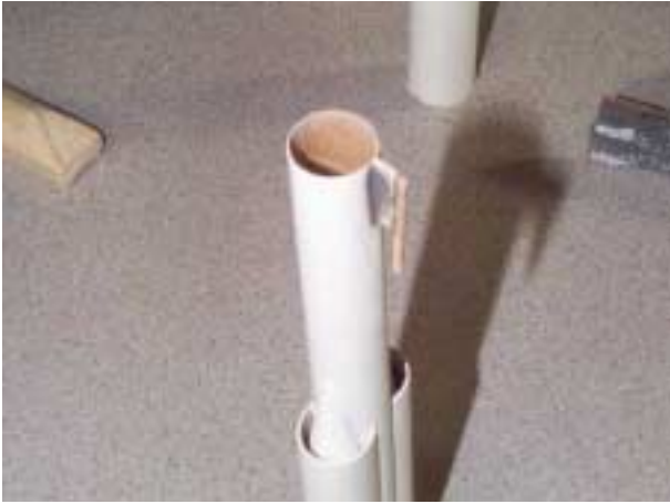
Figure 3-9 – Standoff and Forward Mounting Pin
