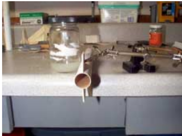
Figure 4-3 – Gluing on Booster Fins
