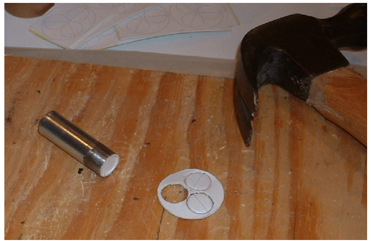
Punching Holes with scrap 1/2" steel tubing
